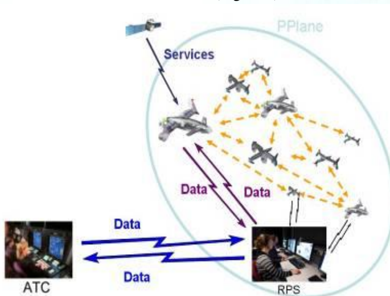
Figure 1: The Personal Plane system architecture concept
